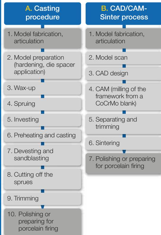
The chemical composition, macroscopic appearance, mechanical and biological properties and processing characteristics in the sintered state are identical in practical terms to those of CoCrMo casting alloys that have been clinically proven for many years.
