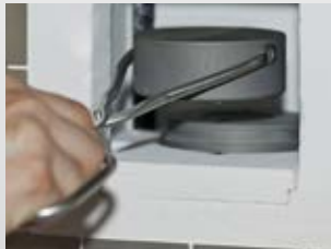
Placing the sinter tray with fitted sinter cover in the furnace
