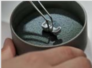
Positioning the restoration in the sinter tray of the Argovent
