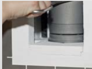
Putting on the sinter retort and starting the sinter process
